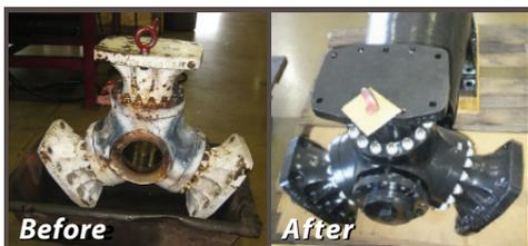
*Fesco Wind Turbine Gear Box Reconditioning*
