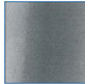
A smooth finish of 16 to 32 RMS\* produced on state-of-the-art precision surface grinders by skilled technicians. This precision ground finish is most commonly furnished. It is ideal for precision layout, gaging, inspection work and facilitates the use of all types of calibration instruments. This finish provides accuracies in tenths of thousandths (.0001") in flatness, straightness, squareness and parallelism. Super finishes of 8 RMS\* or better can be provided at additional cost.
