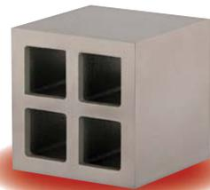
Made from stability treated, quality, close-grained castings and specially designed for the automotive industry, this series is provided with tapped holes for lifting eyes ideal for heavy-duty applications. Precision ground on all six exterior surfaces, these Giant Cube Parallels can be used for parallel and square references in any position. Tolerances are  $\pm .010$  in size, parallel and square to  $.0002$ " in 8". Can be matched pairs.
