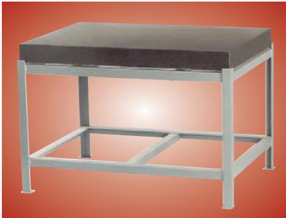
Proper support of granite surface plates is essential to maintain the specified accuracies. All granite plates are finish lapped on three-point support pads and these heavy-duty stands are custom designed to provide the proper three-point support required for each plate.
