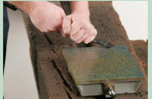
Hand-scraping by a skilled artisan to provide spotting cavities
