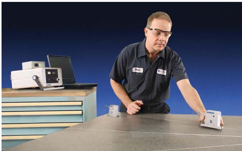
*Robert Kranski, Calibration Technician, inspecting a 48" x 96" x 15" thick Laboratory Grade Granite Surface Plates- using our Talyvel 4 Electronic Level System.*
