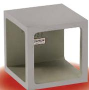
Of similar construction to the 5100 and 5200 Series. BUSCH PRECISION Cube Parallels are **precision ground on all six exterior surfaces to listed dimensions within  $\pm .010$ "**; **opposite sides parallel within  $.0002$ " in 8"** and **with adjacent sides square to within  $.0002$ " in 8"**. The Cube Parallel can also be used as an angle for square references.
