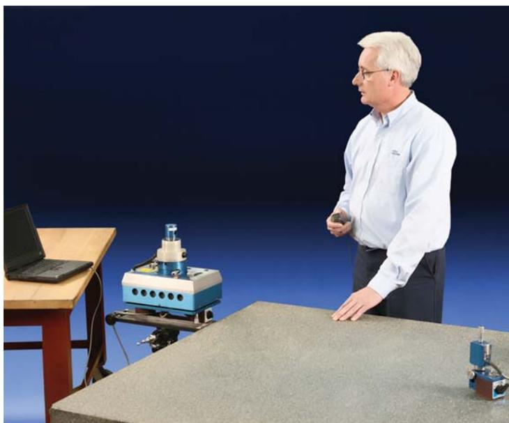
*Peter Gies, skilled Production Engineer, recalibrating a 48" x 96" x 15" Laboratory Grade AA Granite Surface Plates with our Hamar Laser System. This system provides a clear picture of any alignment task, plus documents data in printed form. We verify the most demanding accuracies in flatness, straightness, squareness and parallelism.*
