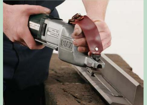
Power-tool scraping to remove initial flakes of metal
